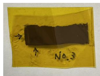
Fig.1 Copper thin film sintered by blue laser
