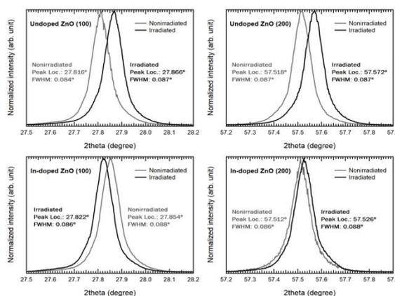
Fig. 1 GIXRD spectra of nonirradiated and gamma-ray irradiated undoped and In-doped ZnO bulk single crystals.
