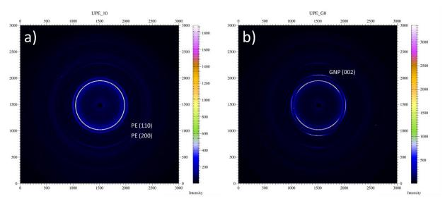
**Figure 1**. Radially integrated Wide-angle X-ray scattering patterns of a) polyethylene and b) polyethylene filled with graphite nanoplatelets nanocomposite (8 wt % loading).
