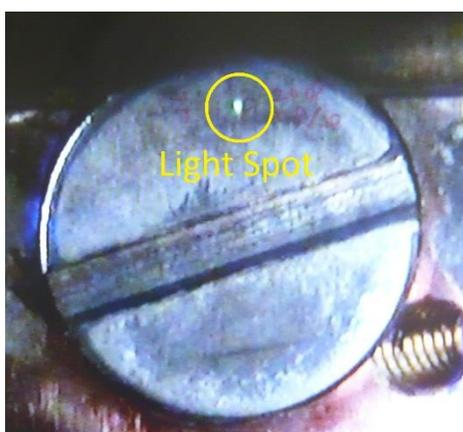
Fig.1 Image of light spot on the sample position. Size of the screw head is 7 mm in diameter.
