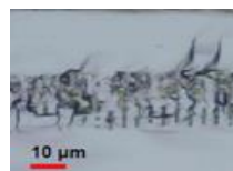
Fig.1 Cross Section of SD layer obtained by optical microscope
