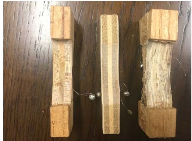
Fig. 2 Specimen (Left: plywood-RLRLR; center: plywood-LRLRL; right: OSB).
