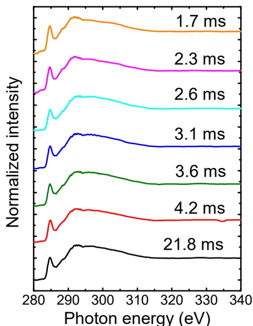
Fig. 1 The NEXAFS C K-edge spectra of a-C films grown with different residence time.
