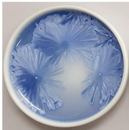
Fig.1  $\text{Co}_2\text{SiO}_4$  添加亜鉛結晶釉
